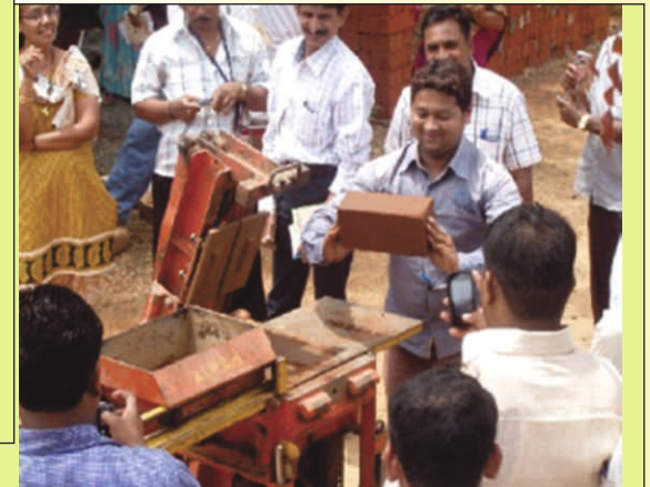
Joy of getting a good quality compressed Earth Block
