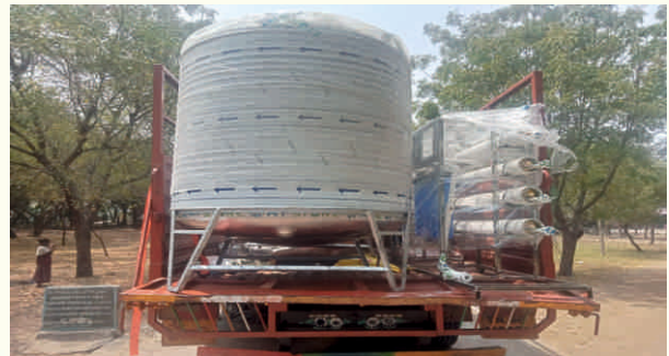
R.O. plant – filter and membrane installation
