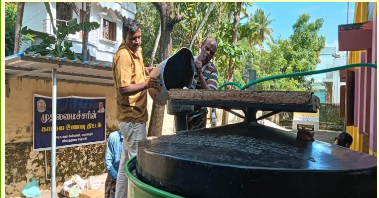
Initial feeding cow dung is on .. to develop bacterial colony
