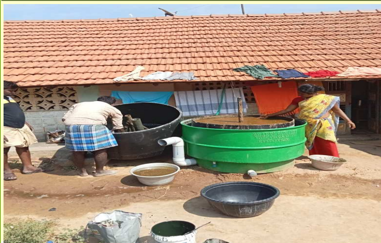
Inlet tank filled with cow dung slurry for the production of microbial colonies
