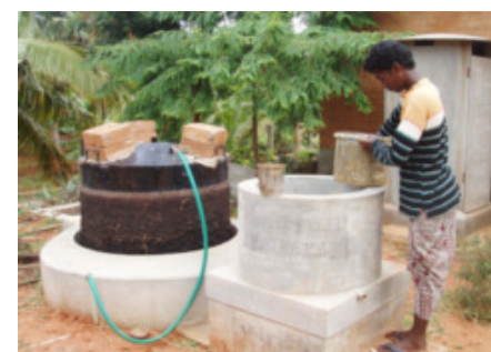
A neem cake based biogas plant at Technology Resource Center of VK-NARDEP
