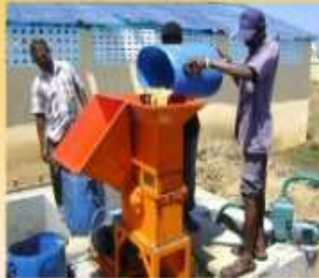
Waste is crushed before feeding
